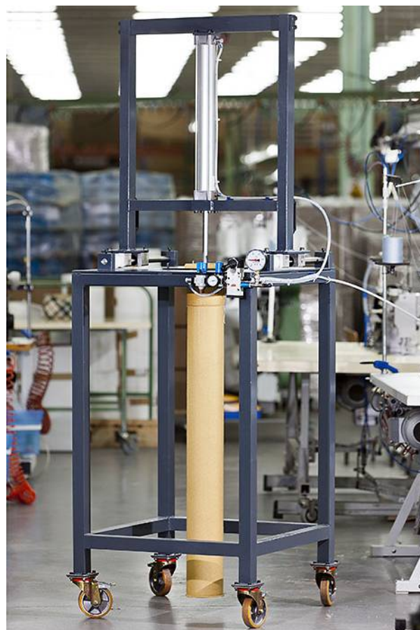
Fitting for hole plate assembly test.
